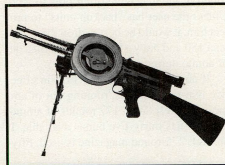
The Ilarco 180 Twin has a capability of firing up to 60 rounds per second with a capacity of 165 rounds.
