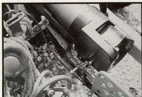
Picture 9: The lanyard is attached to the firing lever (center).
