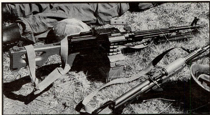
Bulgarian PK GPMG. Note fluted PK-type barrel and reddish plastic skeletonized buttstock. Russian skeletonized buttstock is fabricated from laminated wood. Below and to the right is a Yugoslavian caliber 7.62x39mm M72B1 light machine gun, a copy of the Russian RPK with some minor differences. Photo courtesy of Chris Mayer.
