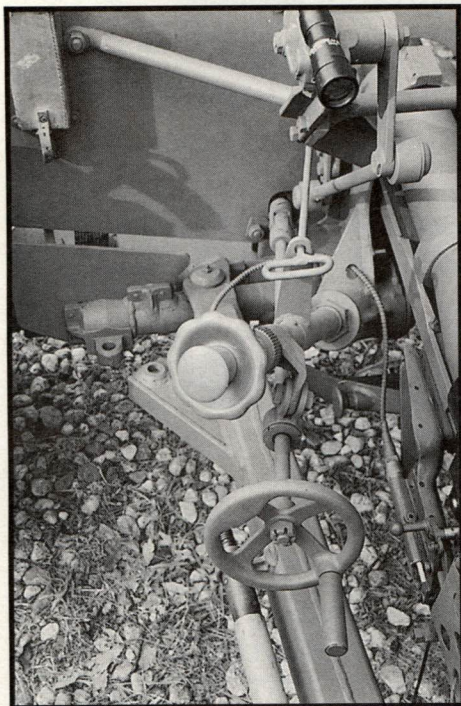
Picture 7: (top-to-bottom): the traverse release handle, traverse knob with firing plunger and the elevation handcrank.
